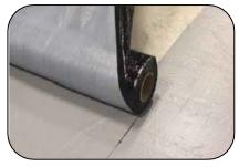
F5 can be used on concrete, plywood, exterior gypsum, DensDeck® Prime, SECUROCK® Brand Gypsum-Fiber Roof Board or other approved substrates in conjunction with Mule-Hide roofing systems. Gypsum decks may require additional securement with mechanical fasteners. Use of AeroWeb, CCW-702 or CCW-702LV is required on all substrates. F5 may be installed directly over a nailed approved modified bitumen base sheet when primed with AeroWeb.
