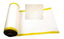
Walkways are required at concentration points (i.e., roof hatches, access doors, rooftop ladders, etc.) regardless of traffic frequency. Walkways must also be installed if regular maintenance (once a month or more) is necessary to service rooftop equipment.
