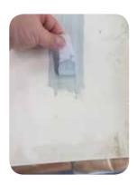
Silicone-based Roof Patch adhesion to aged TPO
