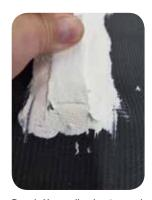
Repair Hero adhesion to aged reinforced EPDM
