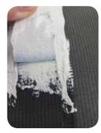
Silicone-based Roof Patch adhesion to aged reinforced EPDM
