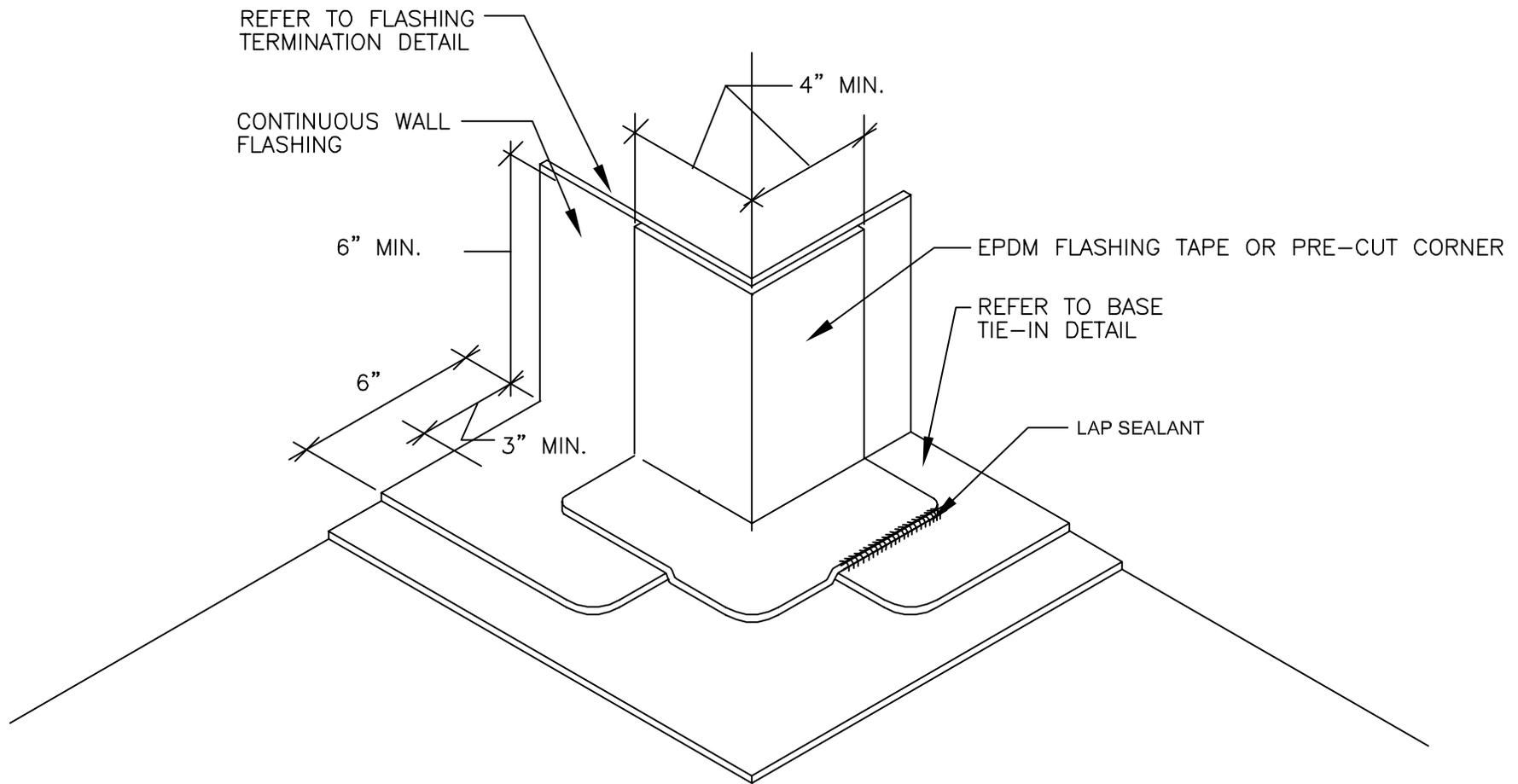
WHEN USING FLASHING TAPES, TAPE PRIMER MUST BE USED
