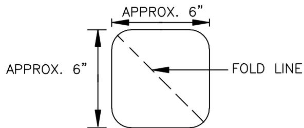
① CUT A SECTION OF NON-REINFORCED MEMBRANE WITH ROUNDED CORNERS OR USE INSIDE/OUTSIDE CORNER; FOLD ALONG LINE AS INDICATED
