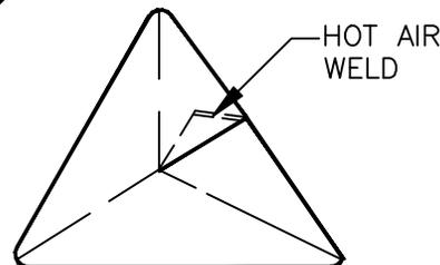
⑥ POSITION AND HEAT WELD CORNER IN PLACE AS SHOWN
