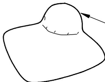
APPLY HEAT TO NON-REINFORCED MEMBRANE AND FORM BY HAND PRIOR TO HOT AIR WELDING CORNER IN PLACE
