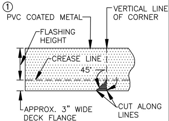
CREASE PVC COATED METAL FLASHING ALONG DASHED LINES AFTER CUTTING AND REMOVING SHADED TRIANGLE.
