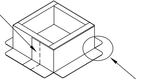
INSTALL PVC UNIVERSAL OUTSIDE CORNERS PER M-H DETAIL MHP-180 OR MHP-181
