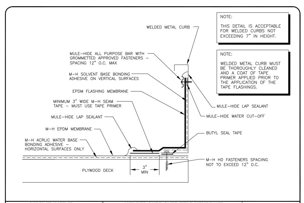
MULE-HIDE PRODUCTS CO., INC. 2010 WELDED CURB OVER FIELD MEMBRANE
