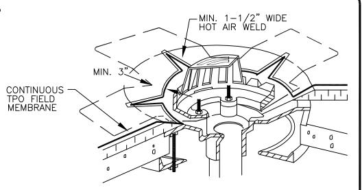
EXTEND TPO REINFORCED MEMBRANE ONTO MEMBRANE SECTION POSITIONED AT DRAIN SUMP AND CUT AS SHOWN TO LAY FLAT IN SUMP. HOT AIR WELD A MINIMUM OF 1-1/2" COMPLETELY SURROUNDING AREA.
