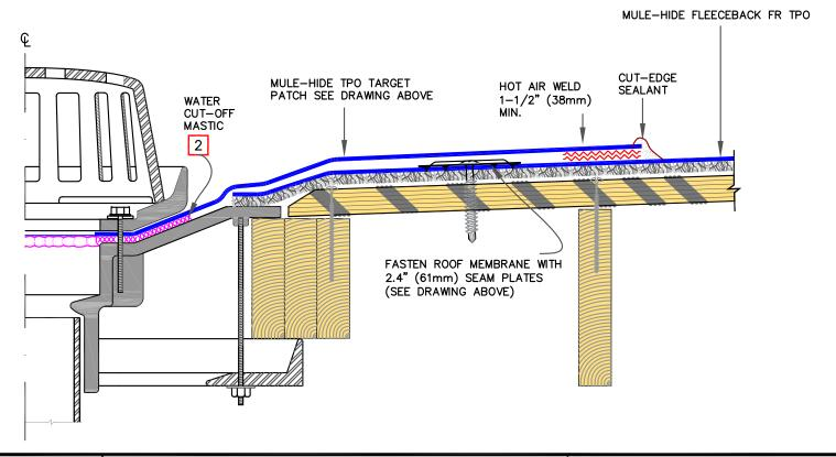
**MULE-HIDE** PRODUCTS CO., INC. DRAIN FLASHING WITH TARGET SYSTEMS:
