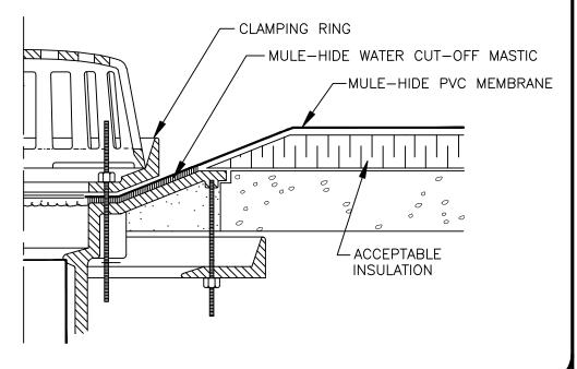
MULE-HIDE PRODUCTS CO., INC. 04/01/2007 ROOF DRAIN FOR DRAIN SUMPS SLOPED LESS THAN 3" PER FOOT SYSTEMS:
