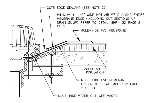
MULE-HIDE PRODUCTS CO., INC. 04/01/2007 ROOF DRAIN FOR DRAIN SUMPS SLOPED MORE THAN 3" PER FOOT SYSTEMS:
