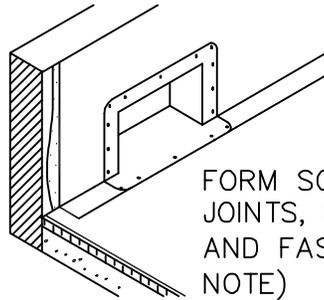
FORM SCUPPER AND SOLDER JOINTS, INSERT INTO OPENING, AND FASTEN FLANGES (SEE NOTE)
