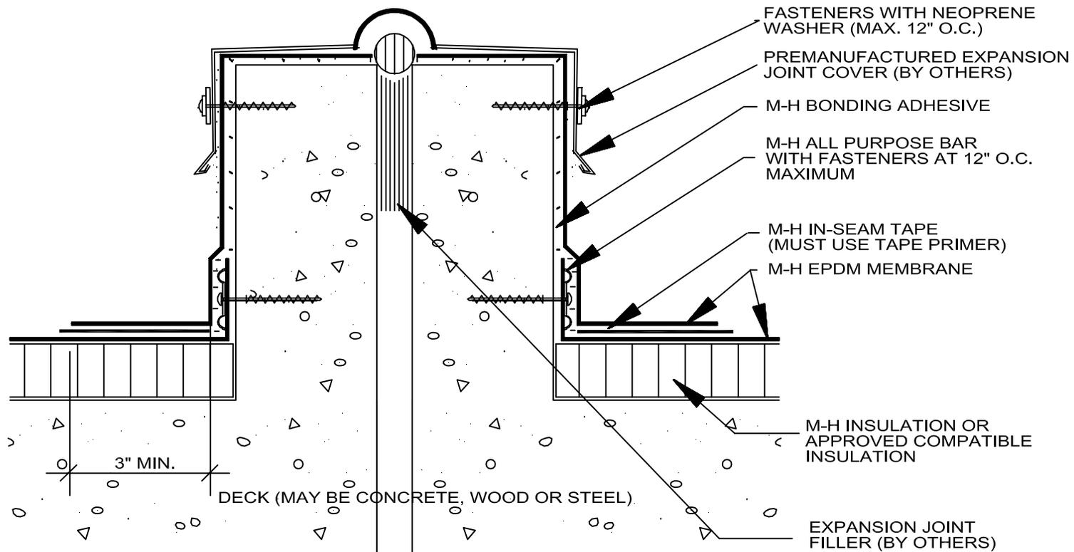
NOTE: DECK AND CURB MAY BE CONCRETE, STEEL OR WOOD.
