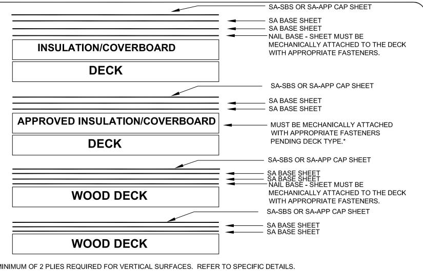
NOTE: MINIMUM OF 2 PLIES REQUIRED FOR VERTICAL SURFACES. REFER TO SPECIFIC DETAILS.
