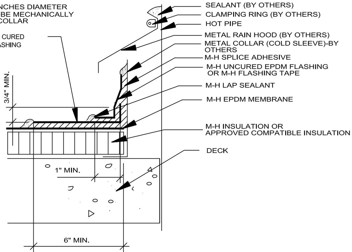
NOTE: IF USING UNCURED FLASHING, PREP EPDM MEMBRANE AND PIPE WITH SEAM CLEANER PRIOR TO
