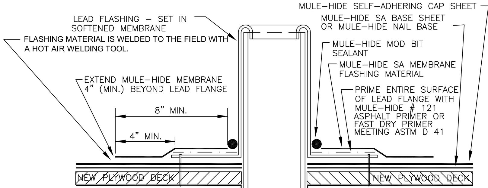
LEAD FLASHING - SET IN SOFTENED MEMBRANE
