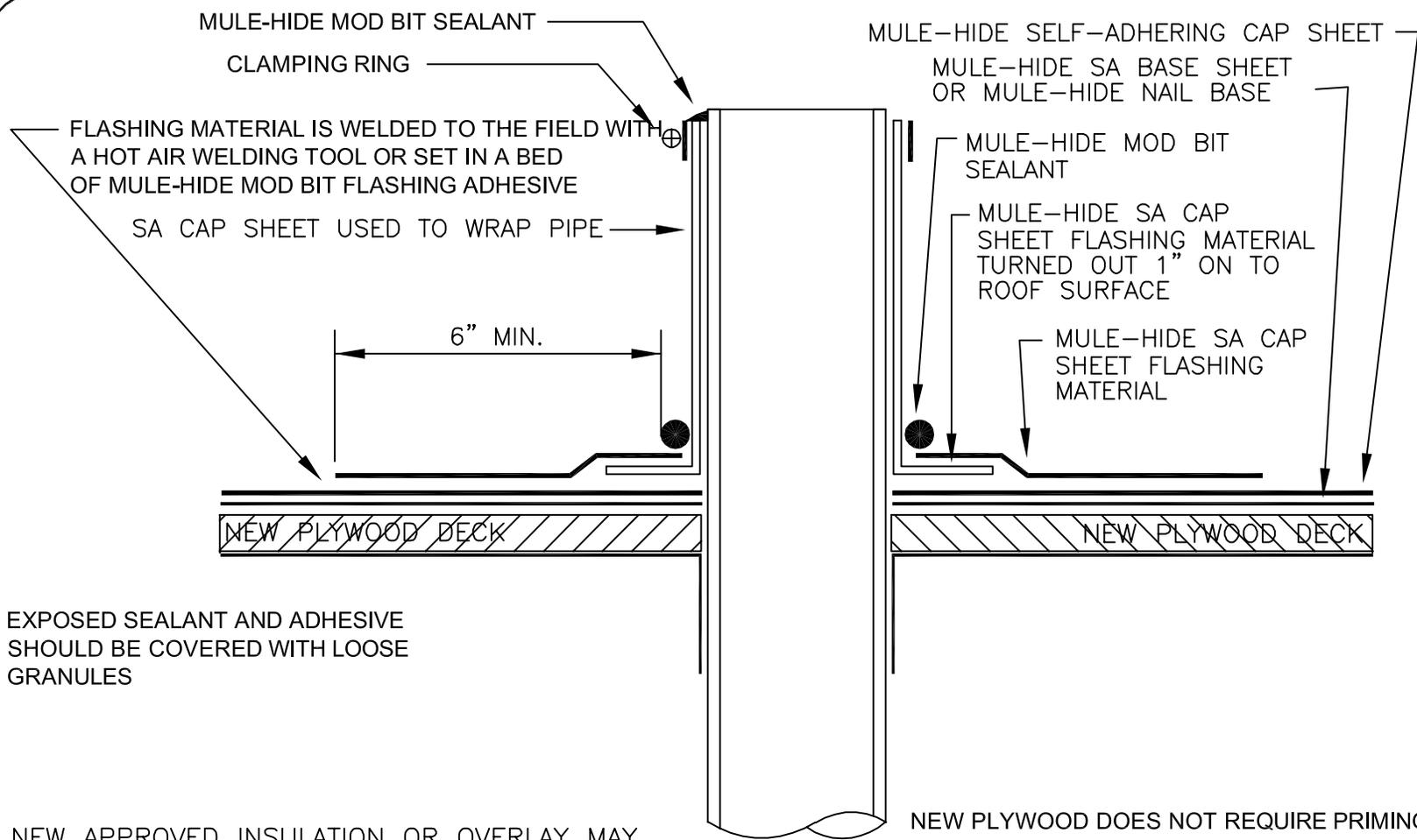
EXPOSED SEALANT AND ADHESIVE SHOULD BE COVERED WITH LOOSE GRANULES
