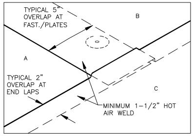
POSITION SHEETS AND HOT AIR WELD THE MEMBRANE A MINIMUM OF 1-1/2".
