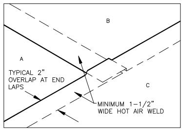
POSITION SHEETS AND HOT AIR WELD THE MEMBRANE A MINIMUM OF 1-1/2" INCHES.
