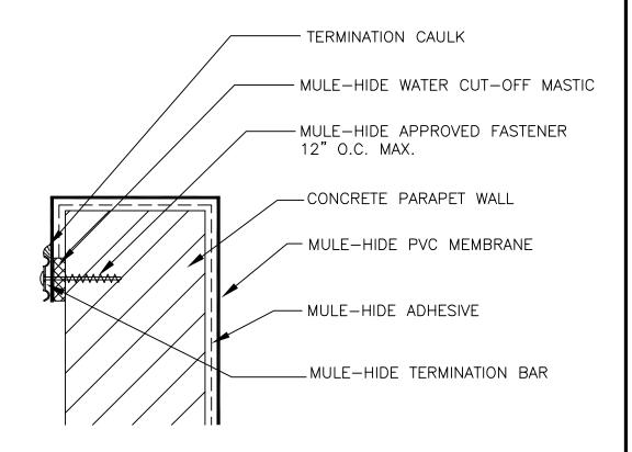
MULE-HIDE PRODUCTS CO., INC. 04/01/2007 CONCRETE PARAPET WALL WITH TERMINATION BAR SYSTEMS:
