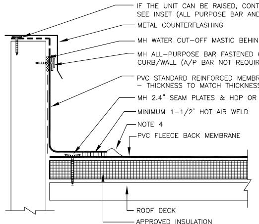
IF THE UNIT CAN BE RAISED, CONTINUE FLASHING TO TOP OF CURB AND NAIL 12" O.C. -SEE INSET (ALL PURPOSE BAR AND WATER CUT-OFF IS NOT REQUIRED)
