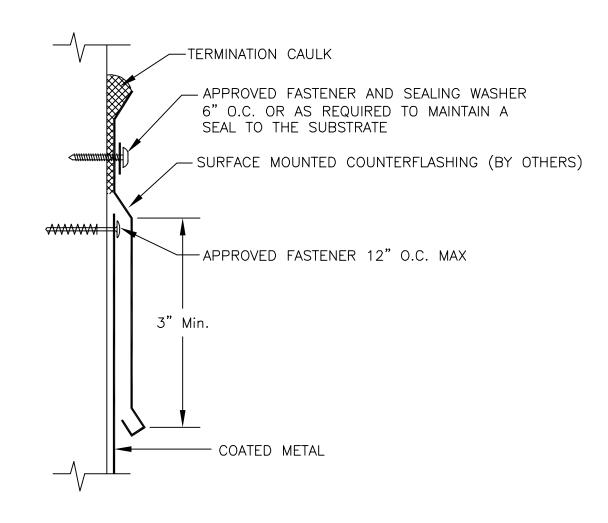
MULE-HIDE PRODUCTS CO., INC. 04/01/2007 SURFACE MOUNTED METAL COUNTERFLASHING SYSTEMS:
