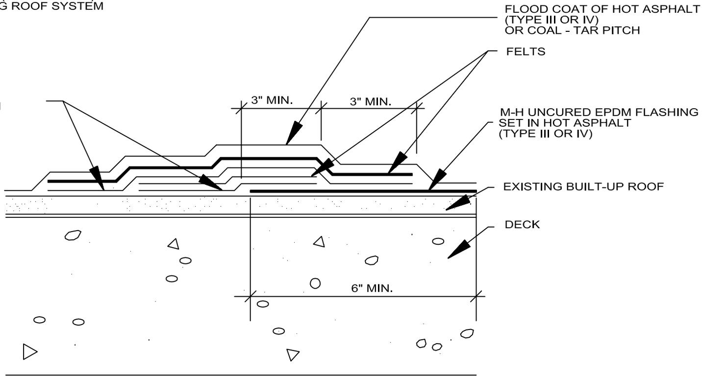
FLOOD COAT OF HOT ASPHALT (TYPE III OR IV) OR COAL - TAR PITCH
